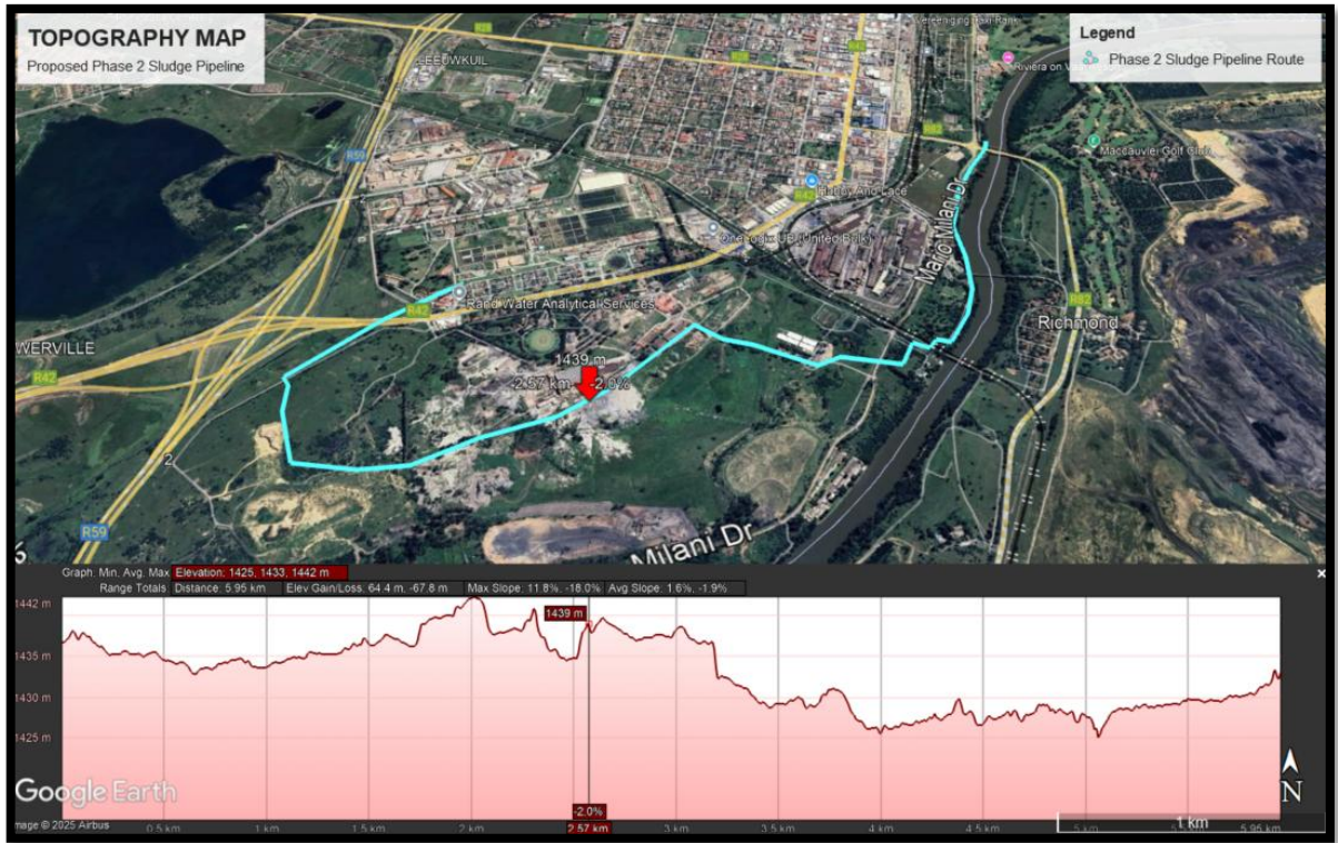
Figure 12: Phase 2 Sludge Pipeline Topography Map
